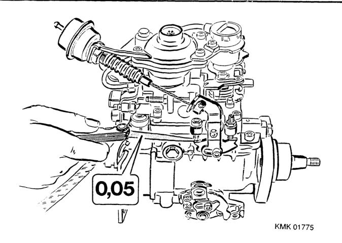
Check dimension "B" (adjusting ring - curved end of basic lever). If necessary, correct dimension "B" by altering position of adjusting ring. Repeat vacuum adjustment test.
